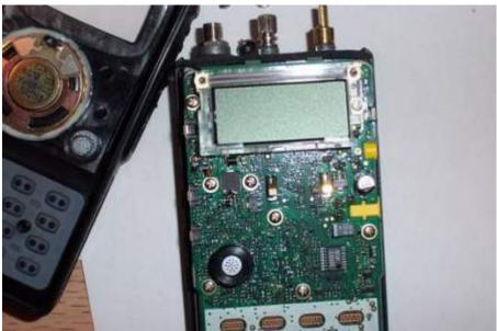
8 Remove R1164. This is found on the right side of the radio, on the board just above the keypad area.
